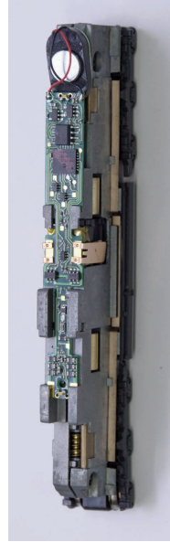
Figure 5: C44-9- 10x18mm speaker in back- frame top modified to fit
