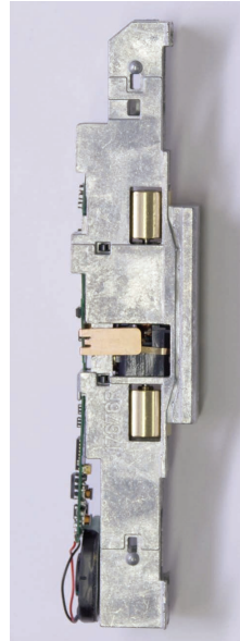
Figure 6: SD70ACe- 10x18mm speaker in upper rear.
